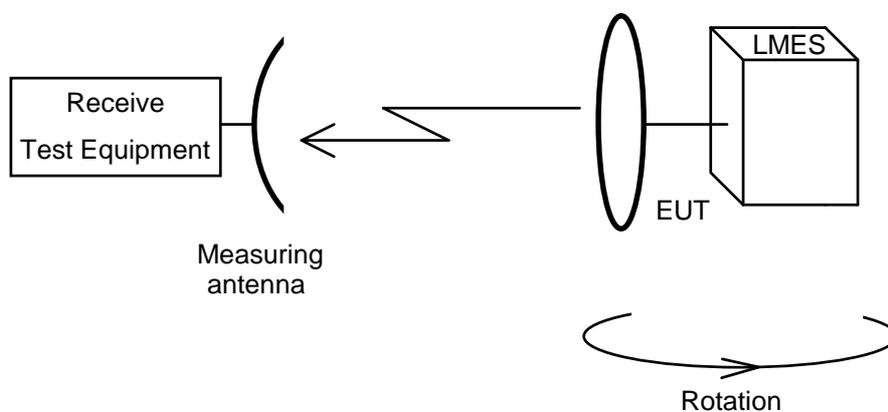
**Figure 3: Test arrangement - emissions measurement, second axis**
