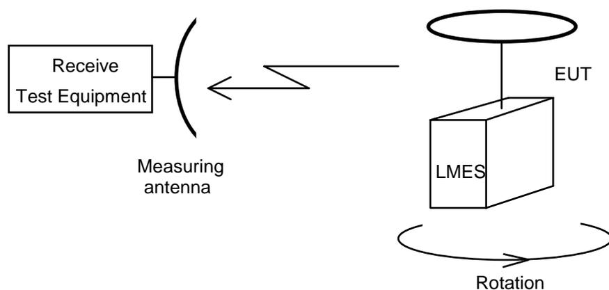
**Figure 4: Test arrangement - emissions measurement, third axis**
